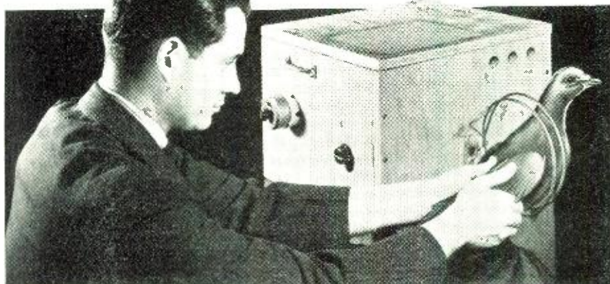
In the experiments, the pigeon was placed in the radio field coil of a small transmitter. In war times the enemy might be able to attract our pigeons over to their side by short wave beams.
