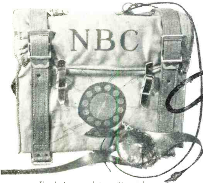
The shortwave pack transmitter used by NBC for parachute work.
